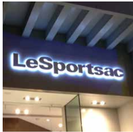
Wall Mounted Sign: Halo Illuminated Reverse Pan Channel Letters
