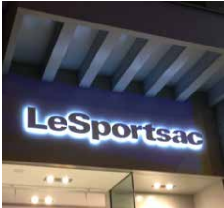
Wall Mounted Sign: Halo Illuminated Stainless Steel Reverse Pan Channel Letters
