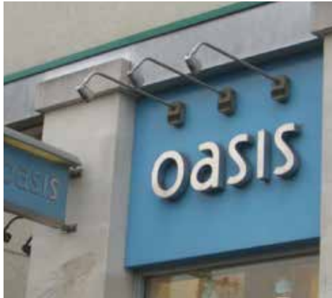
Wall Mounted Sign: Reverse Channel Letters with Indirect (Spot) Illumination
